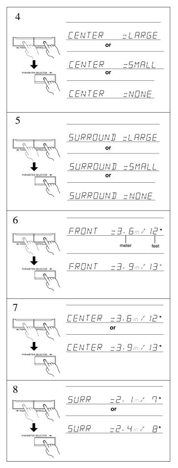
4. Press the PARAMETER SELECTOR▶ button to display the center speaker size parameter, and press the PARAMETER CONTROLLER ◄/▶ buttons to select "LARGE", "SMALL" and "NONE."
